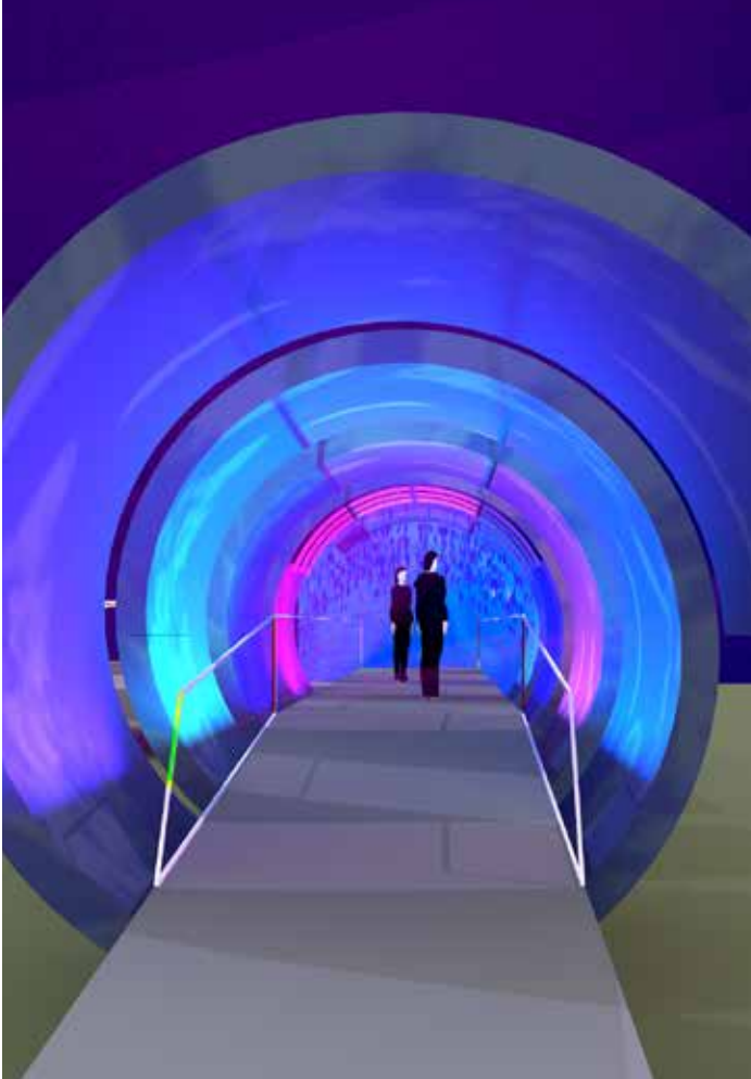
Schulman figured out how to light the tube's interior using basic photometrics and by rendering his ideas, which percolated in Vectorworks Spotlight with Renderworks software.
