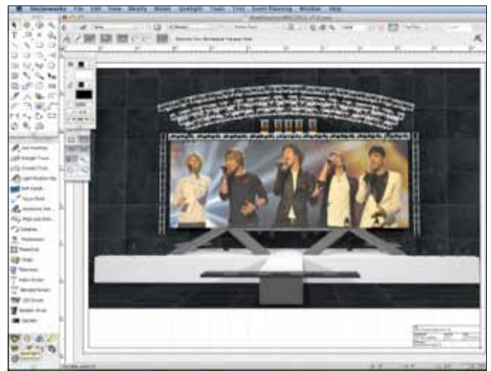
David Lee's fixture placement, seen here rendered in the Vectorworks software, verified that sight lines and fixture selection were coordinated with the 80'x30' video screen.
