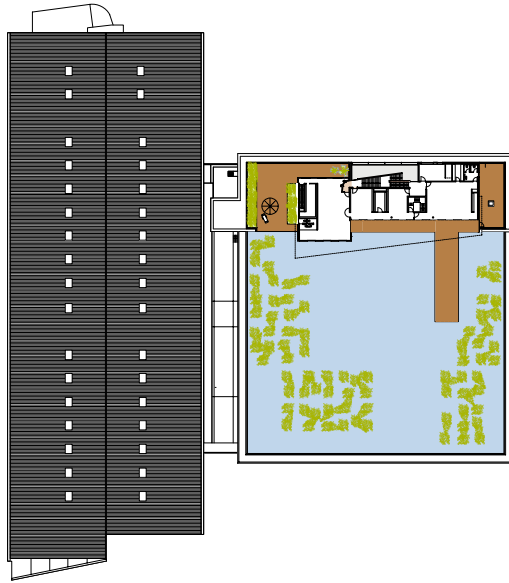
A wooden deck expands as a large wooden terrace, projecting into the 50x60-meter lake with a depth of 15 to 20 centimeters. Image courtesy of BOLLES+WILSON.
